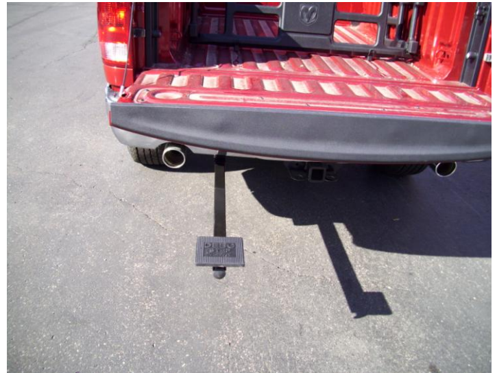
DEBO Step Extended for use with tailgate down.
